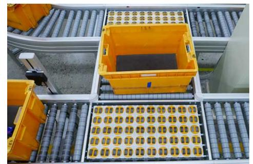
A convincing aspect was the safety of the Avancon system for human contact with the conveyors. A finger protection for each driven conveyor-roller doesn't exist anymore. Here is everything protected inside the conveyor frame - including the drive system and the control system. Nothing sticks out - not even a screw-head. Now the operators are freely working around the Avancon conveyors. The whole conveyor lines are
